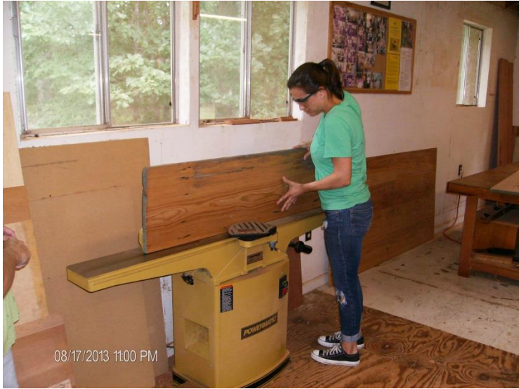
One edge of each board is jointed so it can be ripped to width. Four pieces will be laminated together for each leg.
