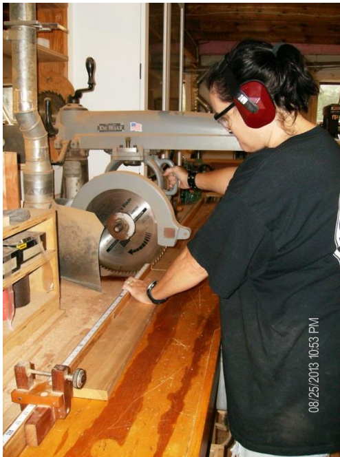
Libba uses the radial arm saw to cut the table aprons to length. Two at 3 ½" x 30" and two at 3 ½" x 66". Then with a dado blade in the table saw, Shana cuts the grooves in the aprons that will receive buttons for attaching the top.
