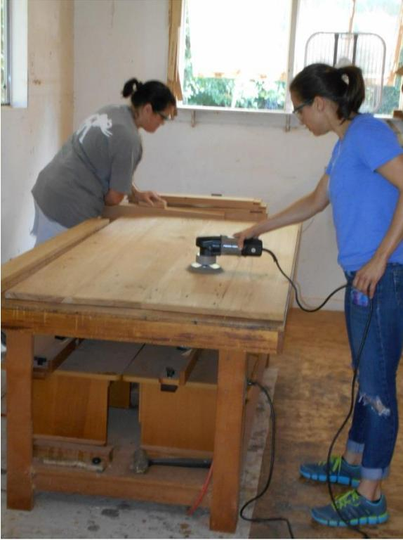
Using a random orbit sander, Shana sands the table top while Libba finishes up the legs and aprons. The next day they apply the first coat of oil finish to all parts. The table has not been assembled yet so as to not take up shop space.
