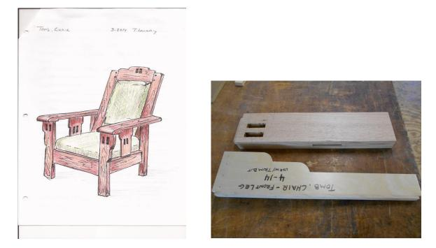
The pattern is cut out and stops are attached so that it will register in the same way to each leg blank. The same pattern is also used to trace the shape onto each blank. The leg is then cut out on the band saw making sure to leave about  $1/16^{th}$  of an inch to the waste side of the line. Note that all mortises and tenons have been previously cut.
