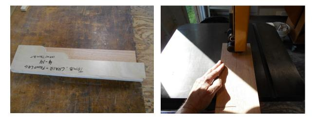
Once the leg has been band sawed, the pattern is attached. I used double stick tape on the bottom end and a screw into the top end.
