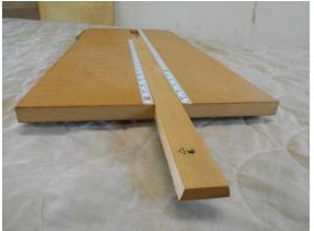
Left photo of the jig shows the guide bar, front stop, lock knob and the slot it travels in. Right photo shows an end view with the adjustable bar extended a little.
