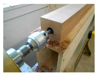
Above are views of the fixture and drill chuck in place and the post being bored. The post is pushed into the spinning bit using the quill on the tailstock. The hole is drilled 2" deep. I'll show more on the complete bedposts at a later date.
