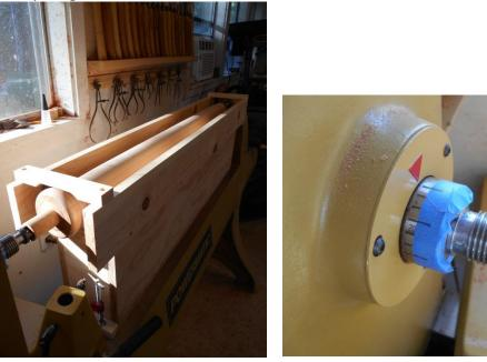
The router is attached to an auxillary base which will guide it along the rails on either side of the turning while keeping it centered. The little blocks screwed to the top of the rails on each end serve as stops to limit travel of the router.
