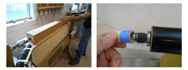
Once mounted on the lathe, the blank is roughed to round and beads and tenon are turned on the bottom end. Corners were ripped off before turning to make this part go much faster and also greatly reducing the chances of corners breaking off while turning.
