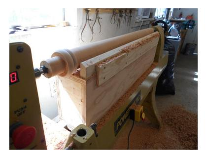
With lathe work done, the turned section can be fitted to the lower section. Now I've got four partially completed bedposts.
