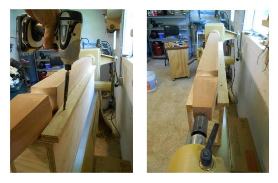
Now with the fixture in place (here's where the accuracy and simplicity come into action) mount the bedpost between centers while it sets on the fixture. If the fixture isn't the right height you'll find out right about now. Assuming everything is OK, you can now attach a strip of wood to the fixture while keeping it along one side of the bedpost. This "fence" will help in keeping each bedpost lined up and stationary as you drill.
