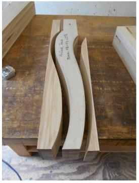
Once the blank has been sawn on one face, tape the parts back together and saw the other face. You can see in the photo at right the leg and all the waste removed.
