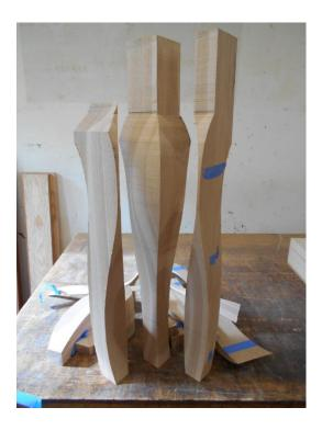
The next two photos show the bandsawn legs. Noticed the mortices were cut before the bandsaw work was done.
