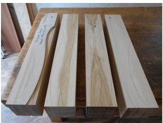
First a pattern is made and traced on the leg blanks. The shape is drawn on two faces at 90 degrees to one another. The back edge of the pattern will touch on what will be the inside corner of the leg. Next I bandsaw to the line.
