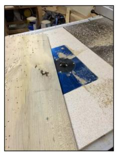
Since my cabinet will need a back it was time to rout out the rabbet along the back edge for the back panels to fit in to. I used a 1/4 inch rabbet bit in the router. I took special care not to route out the of the stop rabbets on the side panels. The next picture gives you a look at those.
