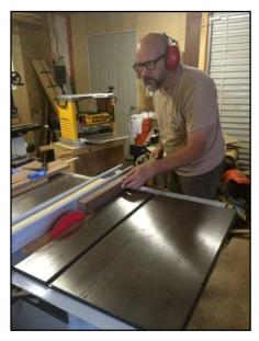
I sawed the leg blanks out of the walnut beam. As best I could I oriented the grain to make the grains more uniform across all the legs.
