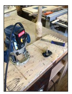
Unfortunately, I forgot to take pictures of most of the next steps in construction—mounting the shelves and divider in dadoes. Fortunately this is not a complicated operation involving only a good router and a clamped straight edge to guide it at 90 degrees. I used a small router plane and a chisel to clean up some of the dadoes as you can see.
