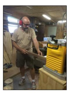
Next, I planed the leg blanks to thickness. I purposefully cut the legs thicker than I needed and then crept up on the final thickness that I wanted.
