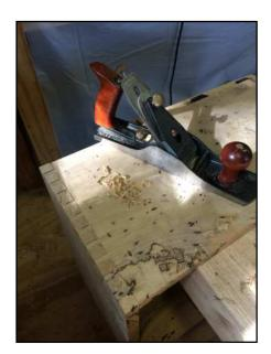
I have to say that the magnolia planes pretty well, but it does tend to powder a little. Here I used a 5 1/2 bench plane to clean up the end grain on the dovetail joints. Note how I am using the end of my bench to support the boards flat while also clamping them firmly in place.
