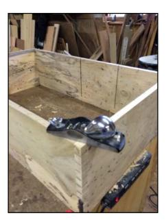
After cutting the joints, I checked for fit. Once I was sure of the fit I cleaned up the corners to insure a very clean edge with a sharp block plane. My alignment was off about a 64th of an inch. The surest and easiest way to bring the case into parallel was to use a plane to square things up.
