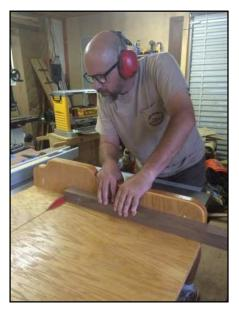
Using a crosscut sled I cut the legs to length. Make sure that all crosscuts are square. A little slip up here and my legs could sit uneven on the floor. Note the mark in chalk on the side face. This is left over from the milling. It was my true face indicator to show the reference face.
