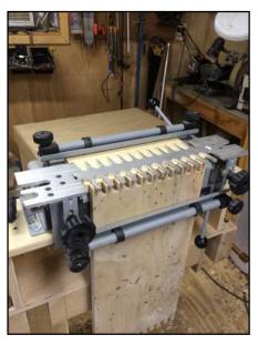
Using a dovetail jig I routed out the joint for the case of the cabinet. The softness and brittleness of the magnolia wood proved to be a challenge since cutting the dovetails tended to cause chip out.
