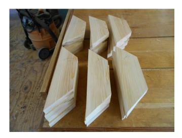
Here's the original covered in almost 100 years of paint. Measurments are taken and parts are cut. It's basically 3 frames stacked one on top the other. Each of the 3 frames are made individually. Two of the frames are then laminated together to be turned on the lathe, the third is left square.
