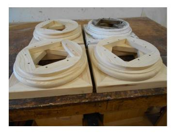
By the way... the originals were just nailed together with square nails and made of cypress so I had to make the duplicates of cypress as well but relied on glue and screws rather than nails. Considering that half of the cutting action on the lathe was uphill in relation to the grain, I was pleasantly surprised that I didn't get any tearout. It's amasing what a sharp gouge can do.
