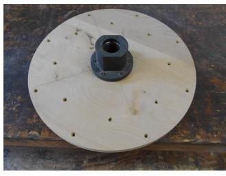
The lathe faceplate is attached to a piece of ¾" plywood. The workpiece is attached and cut on the band saw using the circle cutting jig. Doing it this way prevents me having to remove and re-attach the workpiece from the faceplate, thereby maintaining the same true center from band saw to lathe. With it mounted on the lathe you can see the small hole in the center of the square block which is attached to the faceplate. That is the pivot hole for the band saw circle jig.
