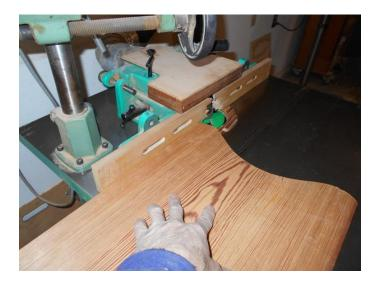
Using a panel raising cutter with a bearing in the shaper, I'm "raising" the panel. I used a template attached to the panel for the shaped top and bottom but installed the shaper fence to do the straight edges. Notice that I am feeding from left to right which is opposite of what you would do on a router table. Because the shaper can run in forward or reverse you can flip and orient the cutter so that it cuts above or below the workpiece.
