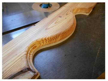
Now with a different cutter, bearing and template I'll shape the molding that will hold the panels in the door. The molded edge is then band sawed off and sanded to the line to fit.
