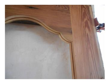
The stiles and rails are cut to size and shape. Mortices and tenons are cut and then, using a slot cutter in the router, a groove is cut in the interior edges of both the stiles and rails. The door is then glued together. The panels go in later.... WHAT? This is actually a pretty old method for making doors and it opens up (get it?) all kinds of design possibilities. The groove receives a spline. The panel sets between the splines and the molding is attached to the splines.
