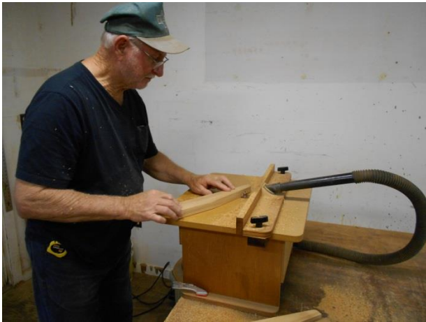
Danny rounds over parts on the router table. Danny, Chris and Terry putting a chair together.
