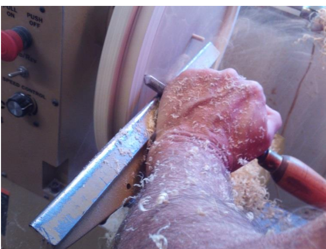
Using the spindle gouge to get the ring close to size.
