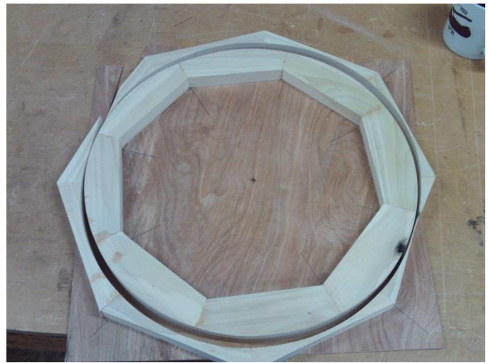
The ring with the waste removed.
