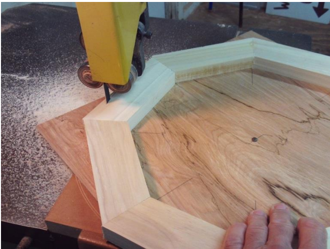
Cutting out the ring using the circle jig.
