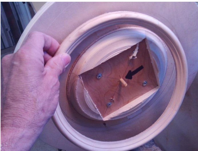
The finished ring pulled loose from the double stick tape and close-up of the molding.
