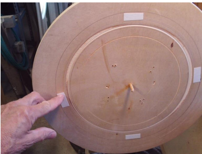
Applying bits of double stick tape and screws. Notice the dowel in the center of the faceplate which fits the same hole used on the circle cutting jig. That hole now centers it on the lathe.
