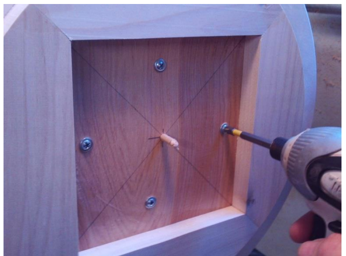
Applying bits of double stick tape and screws. Notice the dowel in the center of the faceplate which fits the same hole used on the circle cutting jig. That hole now centers it on the lathe.
