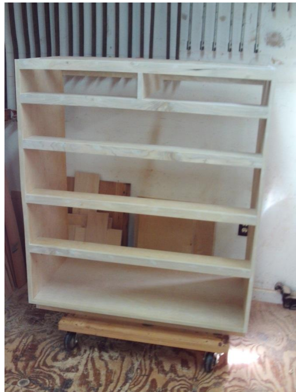
The carcass minus the top and back. They will go on after the drawers have been installed.
