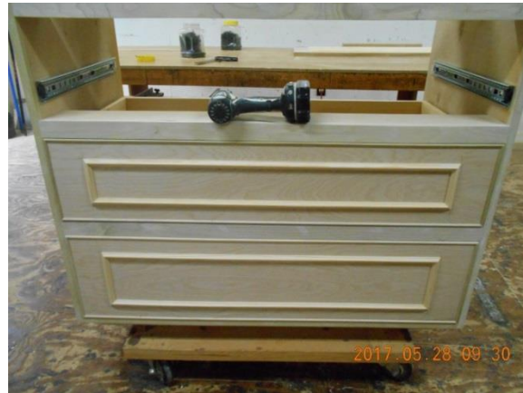
Attaching with screws from inside the drawer and the bottom two fronts attached. This set of cabinets will be painted white and installed in a large closet. They are constructed of birch plywood, poplar and white pine for the drawer boxes. I hope that in reading this you have found it to be of helpful.
