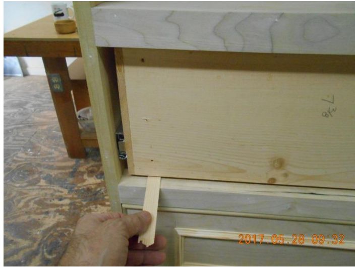
Spacers set in place, one on each end, will locate the front.
