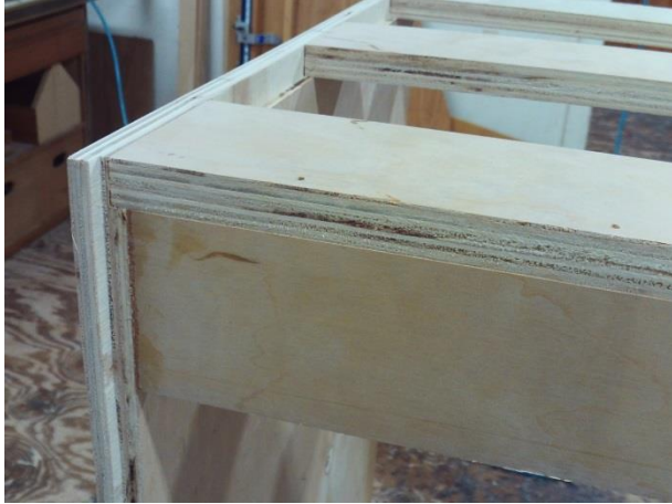
Nailers on top and back.
