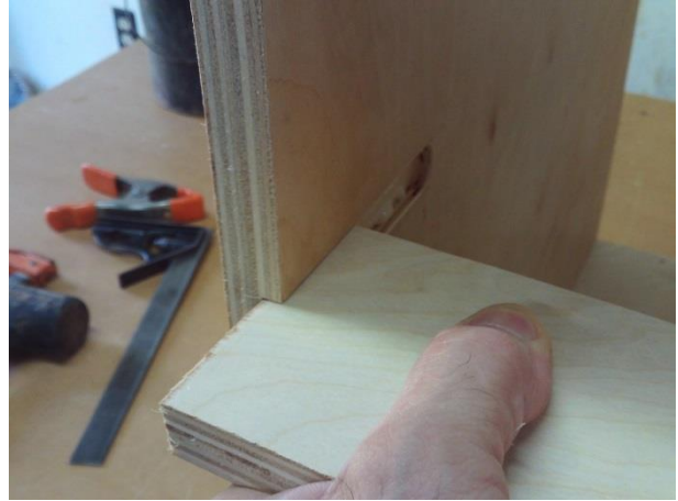
Stiffener for drawer divider going into place.
