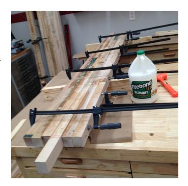
Quick note: Since I wanted to minimize material waste, I used a few shorter boards in the interior of each section and joined them with biscuits end grain to end grain. This took some doing since the ends must be perfectly parallel and jammed together (I used a rubber mallet and a partner). If I were doing it again, I would make all boards the full length.
