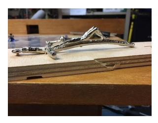
After multiple sandings, last was 220 grit, it was time to stain. I wiped on two coats of stain, twenty four hours apart with a light steel wooling between coats of stain.
