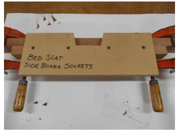
The router template (left) and the template clamped to the ledge (right). The ledge has not yet been attached to the side rail. The dovetails are cut on the table saw using the miter gauge with a stop to locate each slat in proper relation to the blade.
