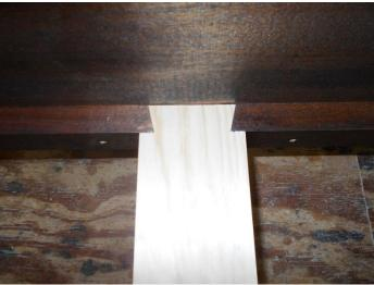
In the process of cutting the dovetails on the ends of the slats and the sockets into which they fit, there is one very important consideration, I want any slat to fit in any location on either bed. In order to ensure that the slats are interchangeable I used a template to route the sockets into the ledges.
