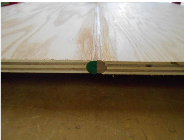
When the glue has dried, the excess is ripped off leaving a nice seamless joint.
