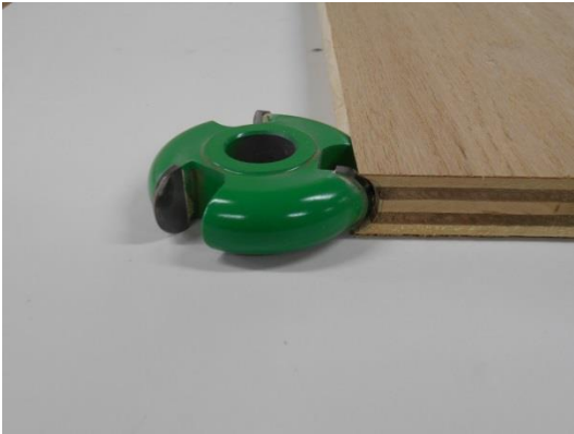
Cove is cut on the plywood.
