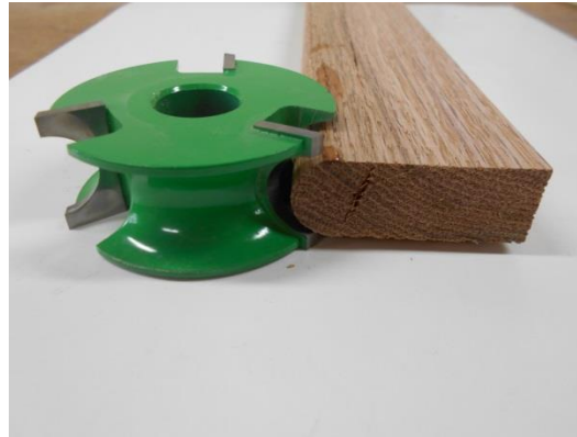
Bead is cut on the oak. This will be the edging.
