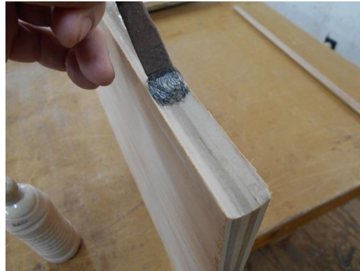
When the glue has dried, the excess is ripped off leaving a nice seamless joint.
