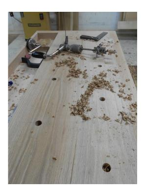
Next I made the vise and fitted it to the bench making certain that everything lined up. Once the glue had dried I then trimmed the excess off the top end of the vise jaw.
