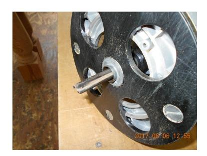
I then locate the center of the hole needed in the workpiece. Using the waste from the template and a ¼" drill I can then line up the template with that center mark.
