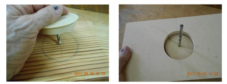
The template is held down with double stick tape. The disc and drill bit are removed. The router bushing follows the inside of the template while the router bit cuts the hole. Notice the offset between the template and the hole in the workpiece. When using bushings you want to take into account the difference between the bit diameter and the outside diameter of the bushing. In this case, to get a 3 inch hole the template needed to be 3 ¼" in diameter.
