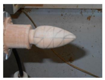
With guide lines in place, It's time for the carving gouge. It's finished up with round rasps and sandpaper and a small tenon is turned on the bottom end.
