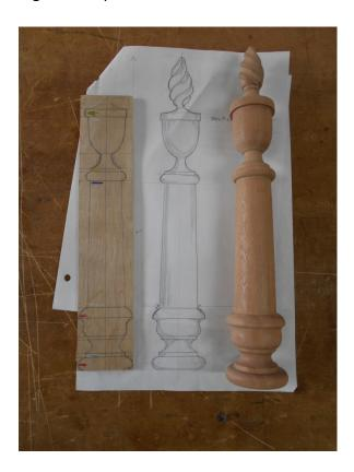
The 1 ¼ inch square blank is mounted into the chuck, turned round and then to a sort of plumb bob shape.
