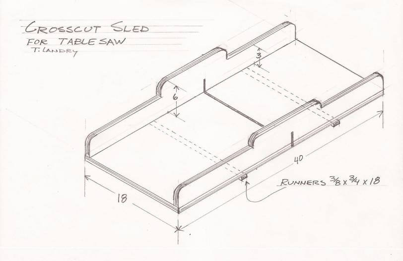
A crosscut sled is a very useful fixture in any shop but its not limited to right angle cuts. By clamping or screwing attachments to it you can cut other angles, tenons or miters. Use whatever scrap materials you have on hand. I usually use ½" or 3/4" plywood for the base, 3/4" plywood for the fences and maple or oak for the runners. You should adapt this plan to fit your saw and the work for which you intend to use it.
