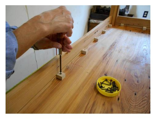
The leg and apron assembly is centered onto the top and attached with shop made buttons. No glue used here so as to allow wood movement in the table top.
