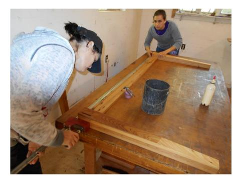
The glue is allowed to cure and the next day the short aprons are glued and clamped into place.
