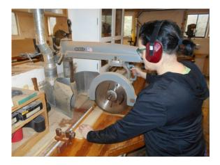
Libba cuts dados at the table saw and cuts parts to length at the radial arm saw.
