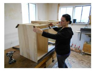
Using glue, nail gun and clamps, the cabinet is assembled. Wood edge tape is applied to all drawer parts and the the drawers are assembled.
