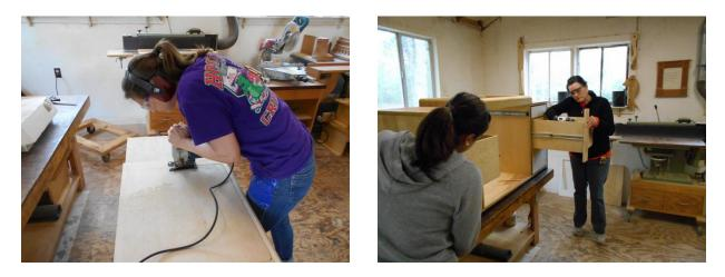
Libba finished the vanity with shellac and paint and it is now ready to be installed. She now cuts holes through the cabinet back for plumbing and appliances and then attaches it to the wall.
