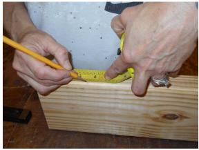
Shana cuts out the tapered legs at the bandsaw and the leg locations are marked on the edges of the saddle. The bevel is used to lay out the angle. The notches to receive the legs are cut using saw and chisel. (this is a good exersize in the use of both)
