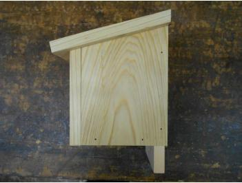
Front and side views. Note the screw bottom center of the front. That screw holds the front on and allows removal for cleaning. (no hinges required)
