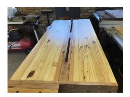
sometimes collaborator into a roubou style. The It has 2 maple inserts, that have a 3/4" wide slot also be raised as high as inserting a spacer vise side of the top is 12 is 11 1/2" wide. There is a glued and dowelled to width of both parts of the
