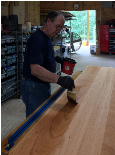
Keith brushes on the sealing coat. Notice the painter's cut can. Easy to hold and has a disposable liner.
