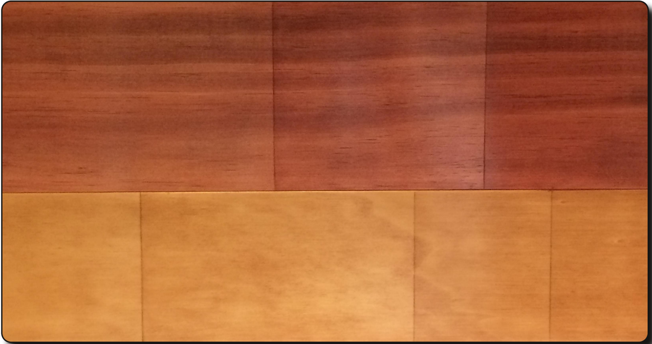
Top: Radiata Pine, Bartley Pennsylvania Cherry, 1, 2, 3 coats Bottom: Pine veneer plywood, Minwax Cherry, 1, 2, 3, 4 coats
